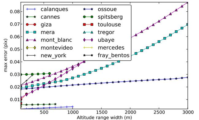
(b) Influence of the width of the altitude range. A tile of size fixed to  $1000 \times 1000$  pixels was selected in the reference image. Virtual matches between this tile and the secondary image were computed using an altitude range of width ranging from 100 m to 3000 m.
