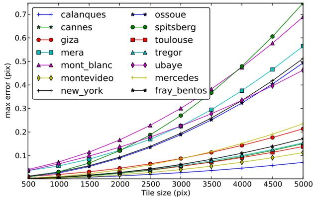
(a) Influence of the tile size. A tile of size ranging from  $500 \times 500$  to  $5000 \times 5000$  pixels was selected in the middle of the reference image. Virtual matches between this tile and the secondary image were computed using an altitude range of width fixed to 2500 m.
