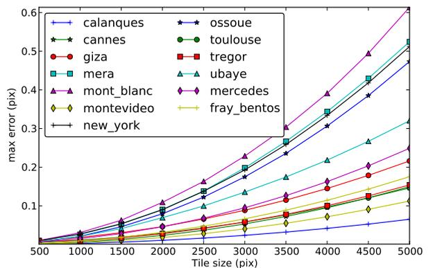
**Fig. 4:** Dependence of the epipolar error with the tile size. A tile of size ranging from  $500 \times 500$  to  $5000 \times 5000$  pixels was selected in the middle of a Pléiades reference image. Virtual matches were computed using the altitude range given by SRTM data. Spitsberg is located outside SRTM domain, thus omitted here.
