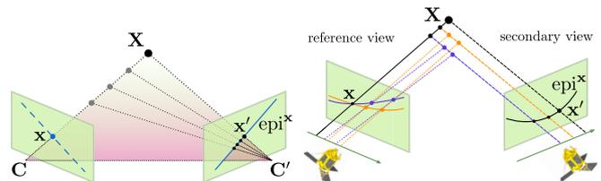
**Fig. 2:** In the pinhole case the epipolar plane defines a correspondence between epipolar lines. In the pushbroom case the projection of a 3-space ray on the secondary view generates a ruled quadric. The projection of this quadric on the reference view contains many epipolar curves: epipolar curves are not conjugate.
